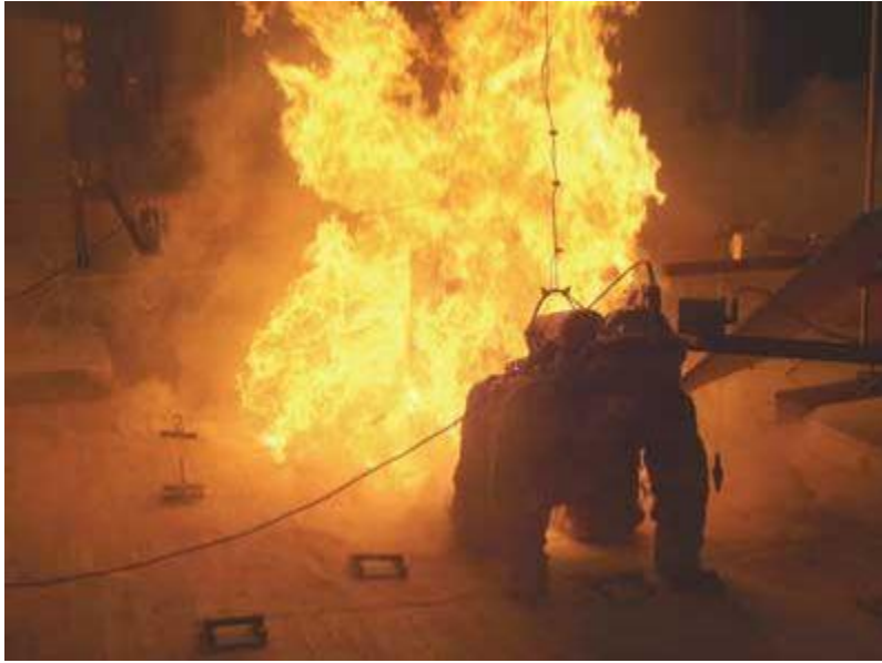
(1) A standing firefighter mannequin is engulfed in flames as he falls through the floor assembly behind the crawling firefighter mannequin. (Photos courtesy of authors.)
