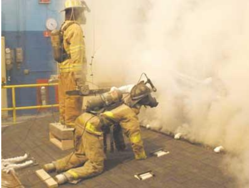
Modern lightweight metal gusset truss roof—with ceiling. Collapse Time = 23:15. (7) A significant volume and velocity of smoke during initial portions of the test.
