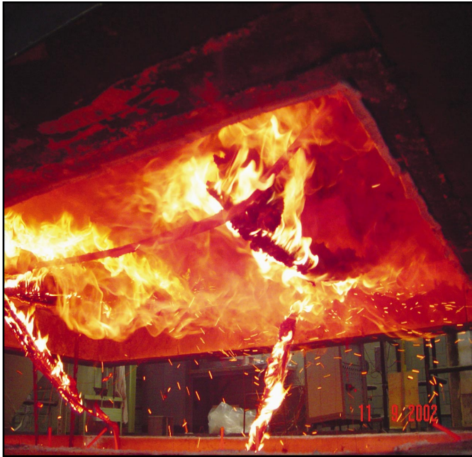
Figure 6: Floor-Ceiling Assembly Removal After Fire Test
