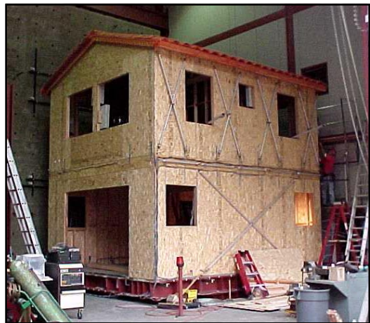
Figure 12 Seismic Test of Walls
