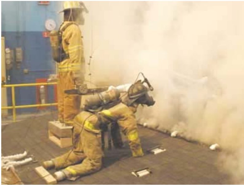
Modern lightweight metal gusset truss roof—with ceiling. Collapse Time = 23:15. (7) A significant volume and velocity of smoke during initial portions of the test.
